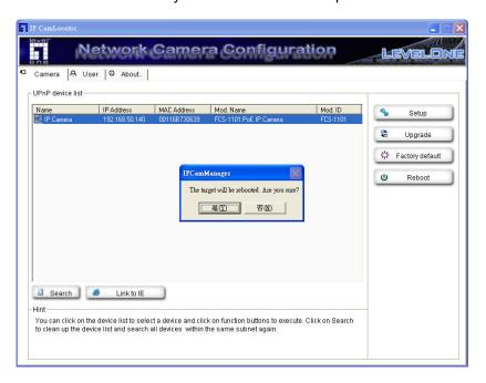
Click on "OK" to continue. The device will automatically reboot after the configurations set to default.
